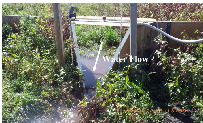
The overland flow of water in a grassed waterway passes through the flume pictured here at the Discovery Farms monitoring site near Brownton.
